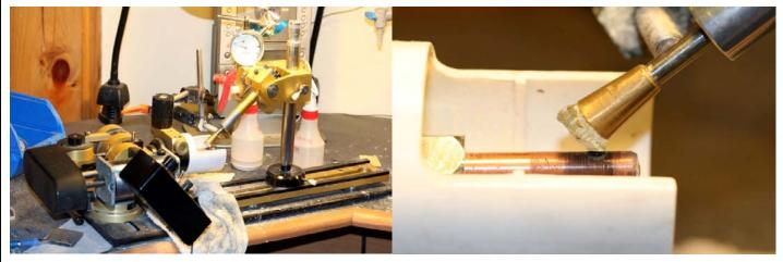
Overall view of the concave faceting machine with doped heliodor.
