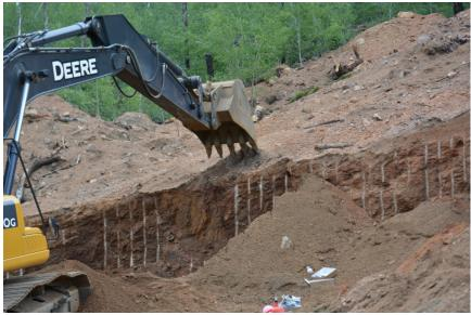
Above left: Drilling lower pegmatites Above right: Reclaimed area just to the north of the Smoky Hawk Left: Tim working the excavator removing wall inch by inch to not damage the pocket by taking any large chunks out of the wall.
